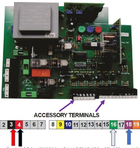
Accessory Terminals 3 & 4 are 24 VAC 1 Amp Output / CP-4 Red (+) and Black (-) connected here.
